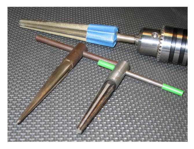
The top reamer in the picture is the reamer I used to ream the taper in the exhaust end of the barrel. The blue tape marks the depth. The reamer with the green handle is the modified handyman's reamer that is used to work the exhaust hole only. The remaining reamer is an unmodified handyman's reamer.
