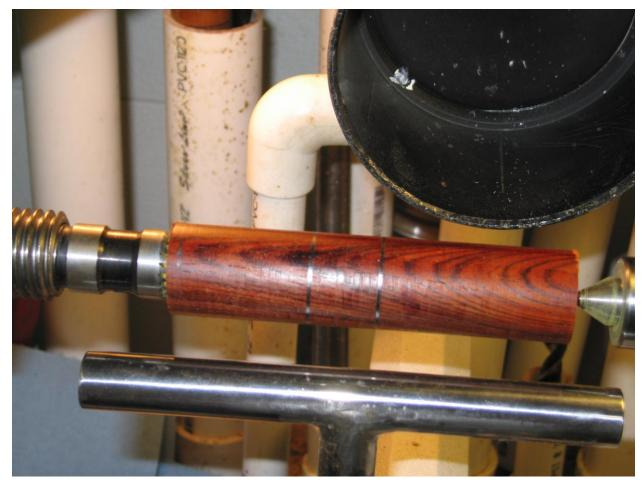
5. Measure 2.200 inches from the exhaust end. Make another pencil mark, place the pencil against the dowel and again roll the lathe spindle to produce a second ring around the dowel. This measurement represents the approximate location of the other end of the wedge. An ideal wedge will measure 0.680 to 0.720 inches in length (front to back) and
